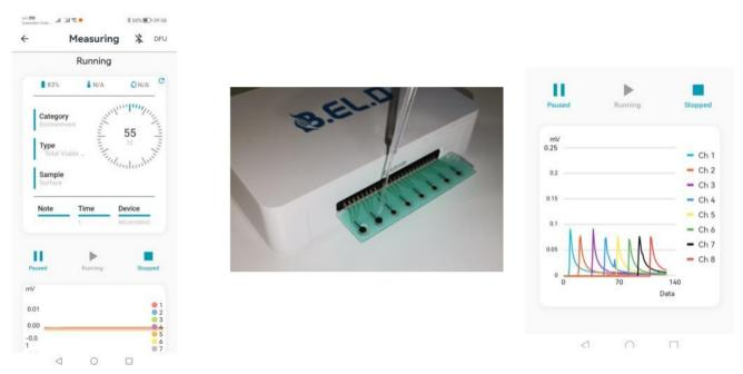
**ATTENTION**, if the lines on the chart do not appear after pressing the start button do not add the sample. Stop the measurement and start it again. Ensure that the lines are visible in the chart and they all start at 0 mV before adding the sample. In case lines do not start at 0 mV stop the measurement and start it again.
