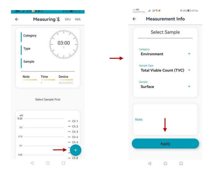
**F.** START the measurement and then add two drops of the sample onto each channel 1-8 with disposable plastic pipette.
