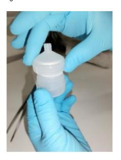
• C. Use the disposable syringe (D) to pass all the water from step A through the filter holder.
