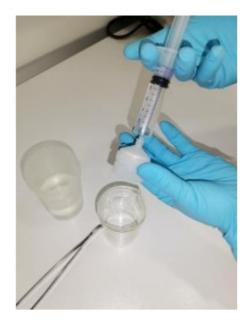
• D. After the filtration, collect the filter with the use of disposable tweezer (F) and place it into the 15ml
