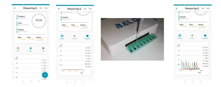
ATTENTION, if the lines on the chart do not appear after pressing the start button do not add the sample. Stop the measurement and start it again. Ensure that the lines are visible in the chart and they all start at 0 mV before adding the sample. In case lines do not start at 0 mV stop the measurement and start it again.
