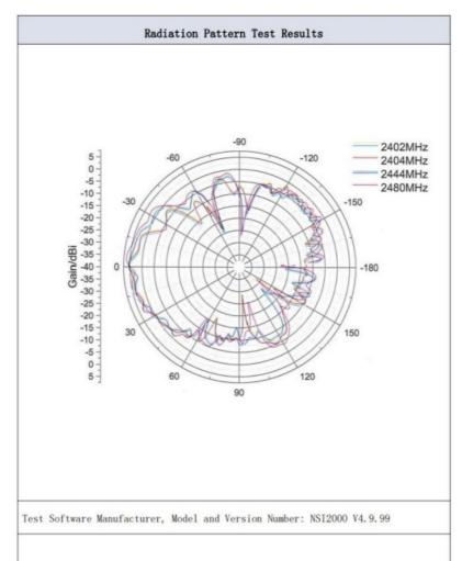
Figure 3.1-2 Multiple connected self-organizing network communication modules Radiation Pattern Test Curve (AUT Horizontal Installation Azimuth Plane 2.402GHz , 2.404GHz , 2.444GHz , 2.480GHz)
