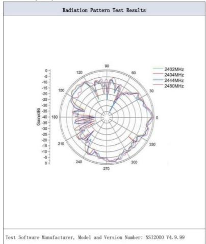
Figure 3.1-1 Multiple connected self-organizing network communication modules Radiation Pattern Test Curve (AUT Vertical Installation Azimuth Plane 2.402GHz 2.404GHz, 2.444GHz, 2.480GHz)
