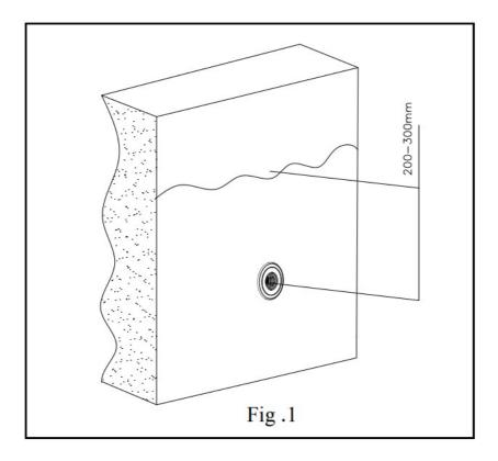
The flow rate required for the installation will determine the number of inlets needed. Three different diameters(14 mm, 20 mm and 25 mm) are available in the eye ball, so you can choose three different flow rates according the pool requirements:
