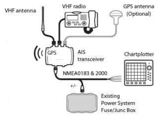
• Switch power on and use the CONNECT-AIS app or PROAIS2 PC Software to program AIS with your vessel information.
