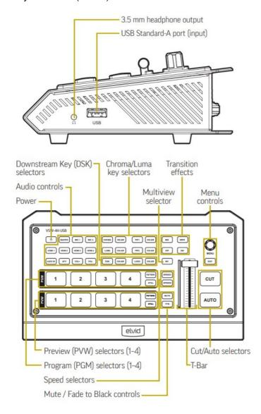
1. Make source and output device connections.
