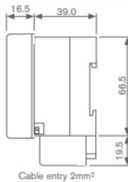
Dimensions for Surface Mounting
