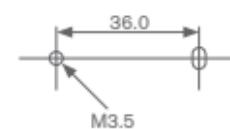
Dimensions for Surface Mounting Adaptor Plate
