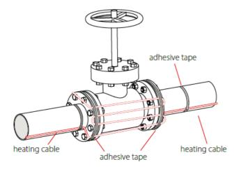
• In areas with large pipe diameters, heating cables must be laid in a loop.
