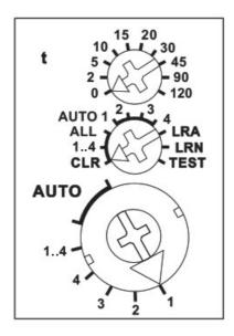
Use the rotary switches to teach-in the buttons and test the 4 channels as required.
