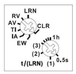
With the top rotary switch in the setting LRN up to 35 wireless pushbuttons can be assigned therefrom one ore more central control pushbuttons. In addition, wireless window/door contacts (FTK) may have a NO or NC function when the window is open. If a direction switch is taught-in, a function e.g. TI can be started using the top switch
