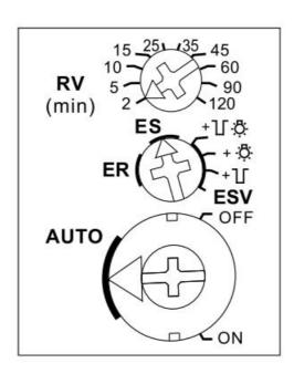
The functions ES, ESV or ER are selectable by means of a rotary switch:
