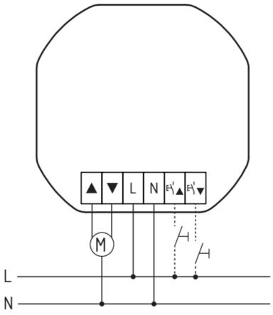
For operation via Apple Home app, make sure that the UP and DOWN directions are connected correctly. These must not be interchanged.
