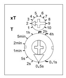
• The LED below the big rotary switch indicates the contact position while time-out is in progress. It blinks while the relay contact 15-18 is open (15-16 closed), and is continuously ON as long as the relay contact 15-18 is
