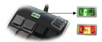
Green light indicates the keypad is work at MOD0 and only upper 4 keys are user defined key (programmed key)
