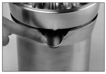
3. With the arm in the down position, remove the Fruit Dome by pressing the button marked EJECT. Let the Fruit Dome drop onto the Juicing Cone.
