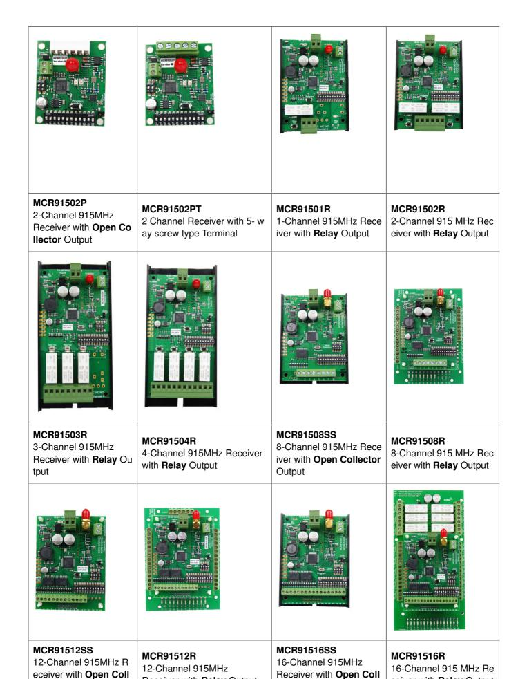
Receiver with Relay Output
