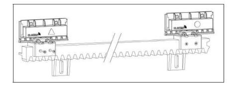
When a steel gear rack is used (or a gear rack that is much slimmer), you will have to use the packing block which comes with the limit switches. Please see the diagram below
