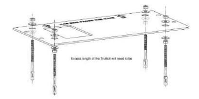
Use TruBolts included in the kit to secure the base plate on the solid concrete surface. Make sure that the distance from both edges of the base plate to the gate should be the same. The excess length of the TruBolt will need to be cut.
