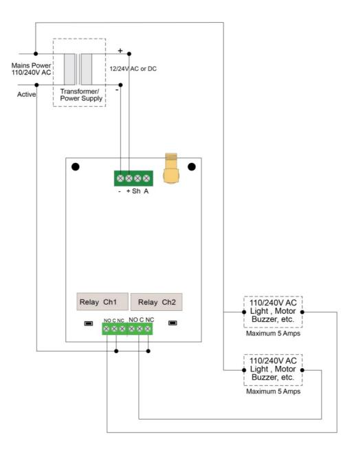
These devices will operate with the Remote Control Transmitter
