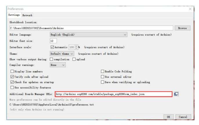
click the menu bar of the Tools – Development Board – Development Board Manager, and then search for "ESP8266" to install the Arduino support package for ESP8266 2.5.2 or the latest version!
