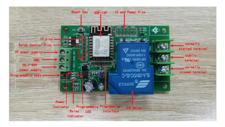
**Burning port:** GND, RX, TX, 5V of ESP8266 are connected to GND, TX, RX, 5V of the external TTL serial module respectively, IO0 needs to be connected to GND when downloading, and then disconnect the connection between IO0 and GND after downloading is completed;
