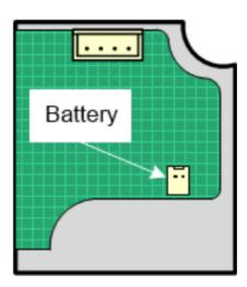
If you need to change the battery or remove it for whatever reason, please disconnect from the connector behind the stainless-steel bracket inside the ERT-A2 as shown in the diagram above.
