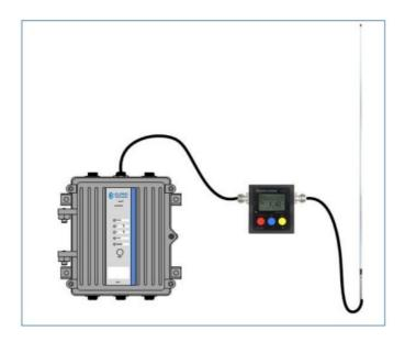
Each connector is clearly labelled, connect the TX to the Transmitter and the ANT to the Antenna or if only measuring TX power a suitable dummy load to accommodate the power level.
