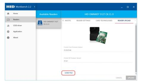
After loading the WBO file, you can compare the firmware version currently installed on the device with the version in the file and decide whether to proceed with the upgrade process.
