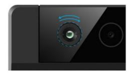
For the accuracy of temperature, please use the Temperature Sensor Pro after turning it on for 5 minutes.
