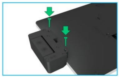
5. Remove the protective film from the included mylar covers and place the covers over the screws.
