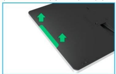
3. Gently press the Temperature Sensor Pro into the peripheral bay making sure the connector is mated.
