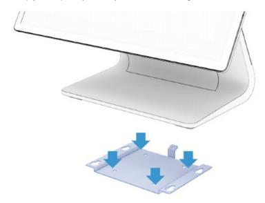
Secure the mounting bracket to the table using the appropriate screw type and length. Elo suggests M4 or #10 screw diameter.
