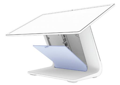
2. Route the DC power cable through the hole in the bottom of the stand and connect it as shown. Connect other I/O cables as needed (see back page) Make sure all cables route through the plastic clip at the bottom.
