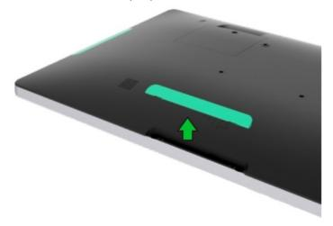
3. Gently insert the status light kit into the peripheral bay taking care to ensure the connector mates properly
