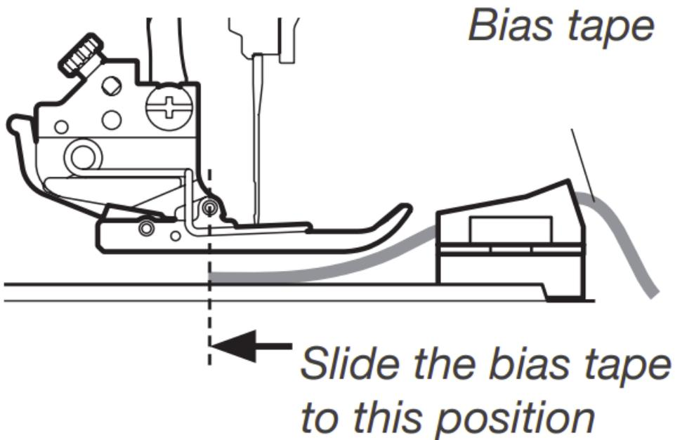
Slide the fabric under the attachment and the bias tape to the rear of the needle drop position.
