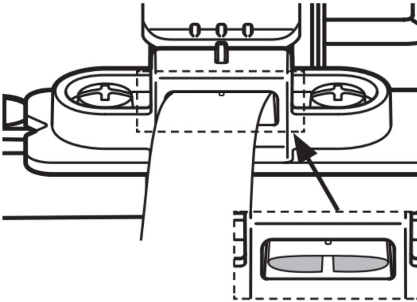
Slide the bias tape under the presser foot to the rear of the needle hole.
