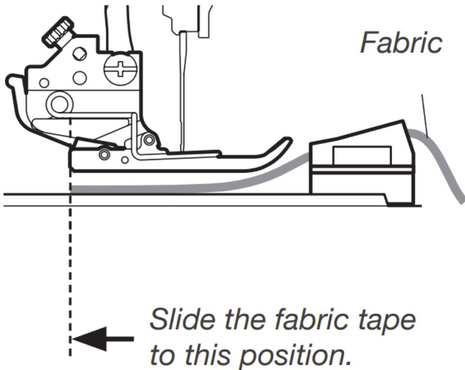
Be sure that the seam lines (left and right) are set at the proper positions for the finished width. Lower the presser foot and start sewing.
