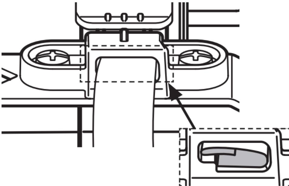
Slide the fabric tape to the rear edge of the presser foot.
