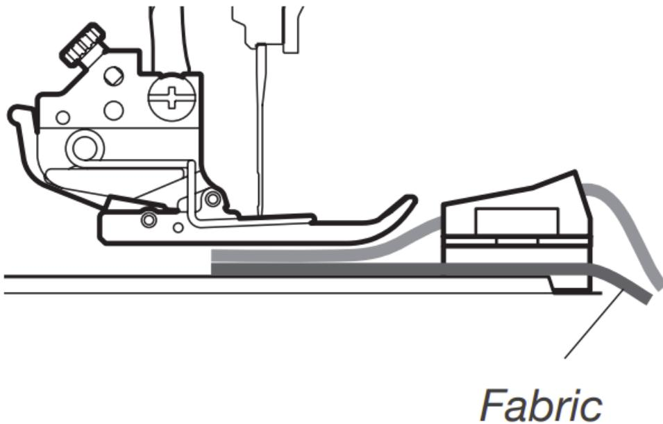
Be sure that the fabric, bias tape and seam lines (left and right) are set at the proper positions. Lower the presser foot and start sewing.
