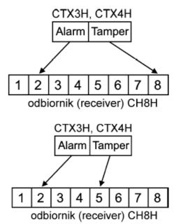
2. Without TAMPER alarm diversion allowing identification of TAMPER alarm source. Learn detector using only its TAMPER switch to any output of a receiver (example: to output 5 of CH8HR.). After learning, TAMPER alarm is active in output 5 while open/close alarming is always signaled three outputs backward, in case of the
