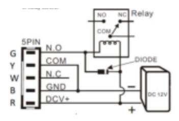
• Connect diode when the control terminal is loaded, to absorb surge and prevent damage to sensor
