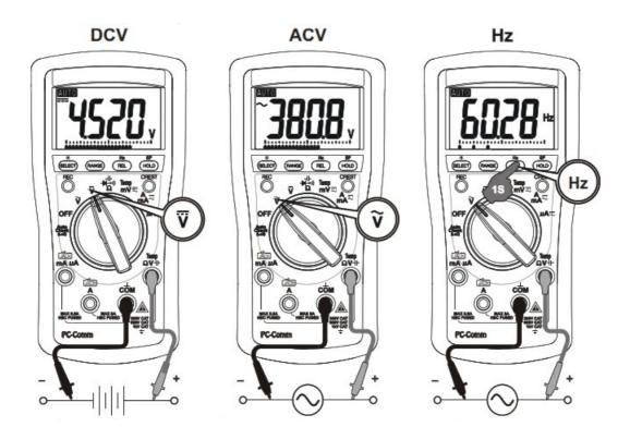
Press the Hz push-button for one second or more to activate or to exit Hz.
