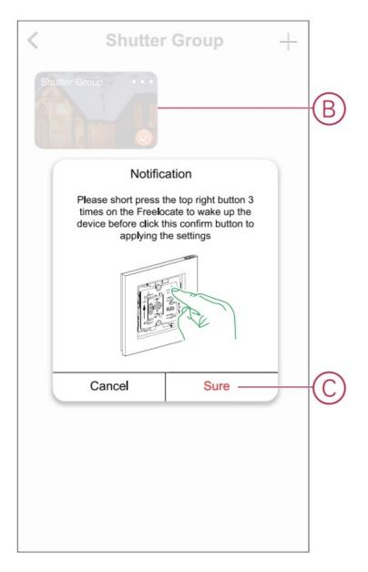
8. Short press the top-right push button 3 times on the Wireless switch to activate the device.
