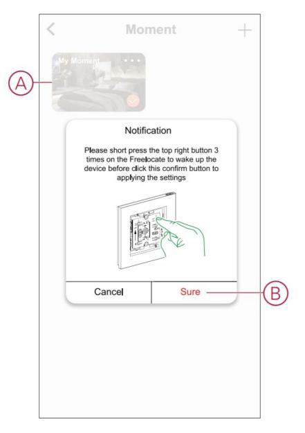
5. Short press the top-right push button 3 times on the Wireless switch to activate the device.
