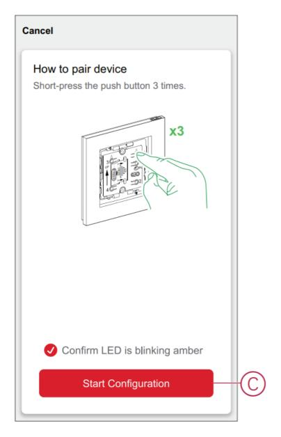
9. After a few seconds, a solid green LED indicates that the device has been successfully paired to the ELKO SmartHUB.
