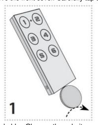
Slide the CR2032 battery into the battery holder. Observe the polarity.
