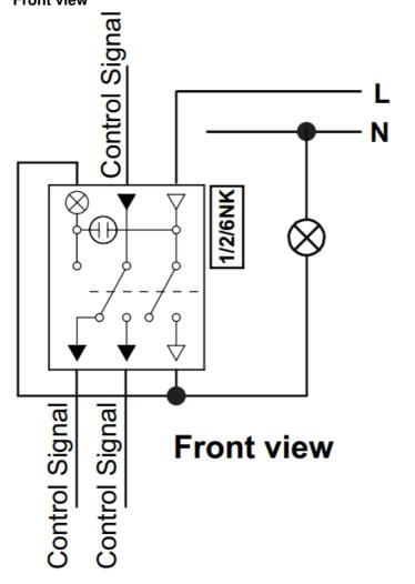
1-pole. Switch light when card is extracted.
