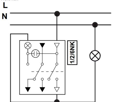
1-pole. Switch light when card is extracted. Separate reverse for Control signal. Front view
