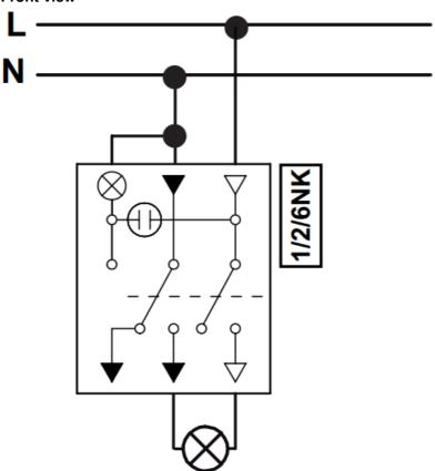
1-pole. Switch light with or without card. Separate reverse for Control signal Front view
