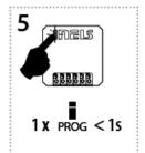
Press of programming button on receiver RFSAI-62B shorter then 1 second will fi nish programming mode. The LED lights
