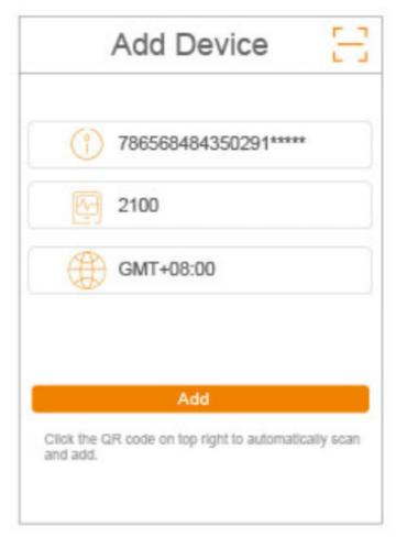
b. Turn on sensor RCW-2100/2200 as shown below. Then sensor will automatically search and connect to any nearby or available gateway. Once it has been connected, sensor(s) will start uploading the real-time data automatically based on your setted uploading intervals.
