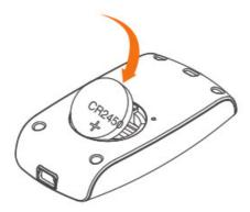
3. Put the cover back and tighten the cover. e)
