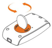
2. Install the battery with "+" side upward and keep it under the metal connector.
