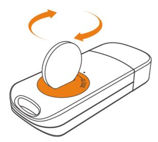
Note: Do not remove the battery when the logger is running. Please change it when necessary. Install Software
