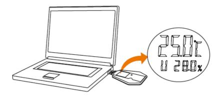
Connect the data logger to the computer via USB cable, and wait until shows on the LCD screen, then download data via:
