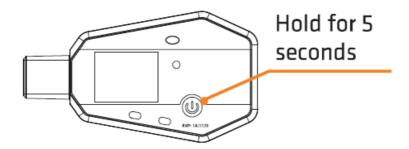
**Press Button\*:** Press and hold the button for 5 seconds until the **■** icon shows on the LCD, indicating the logger stops logging.
