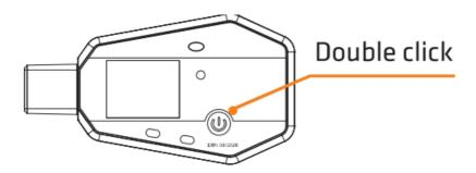
Double click the button to mark current temperature and time, up to 10 groups of data. After the data is marked, the LCD screen will display !MARKI, Log X and (X: current marked numbers).
