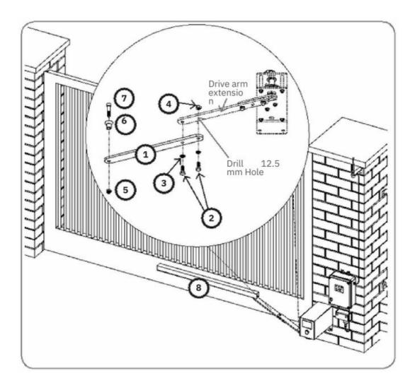
If you have a limited side room, an optional minimum side room kit reduces the gate opener's required side room to the width of the drive unit (135mm). (ATA Order code 90182).
