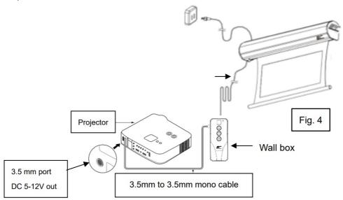
5. Wireless 5-12 volt trigger (Fig.5): Requires a 3.5mm to 3.5mm mono cable (Not included). The Radio Frequency (RF) remote control serves as a dual purpose, independently as a handheld remote control, or as a Wireless 5-12 volt trigger. The radio frequency technology sends a wireless signal that synchronises the screen's drop & rise with the projector's power cycle.
