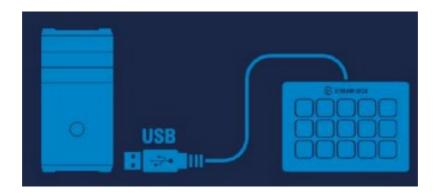
Connect Stream Deck directly to a USB port on your PC or Mac – do not use a USB hub.
