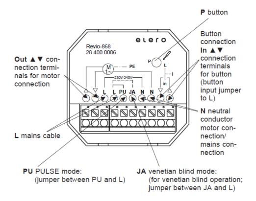
Roller shutter mode: no jumper between L and PU or between L and JA
