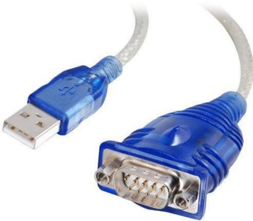
Figure 2 Connector cable USB end (left) and RS232 end (right)
