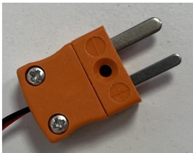
◦ Figure 6 Thermocouple end of Element-B connection cable
