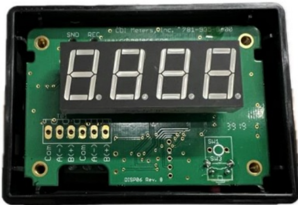
Figure 3a (left): Display board. Figure 3b (right): Output board located underneath the display board
