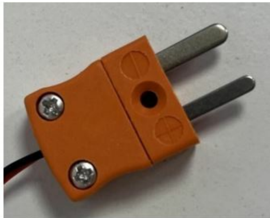
Figure 2 Thermocouple end of Element-B connection cable
