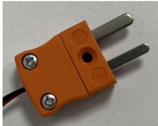
Figure 3 Thermocouple end of Element-B connection cable
