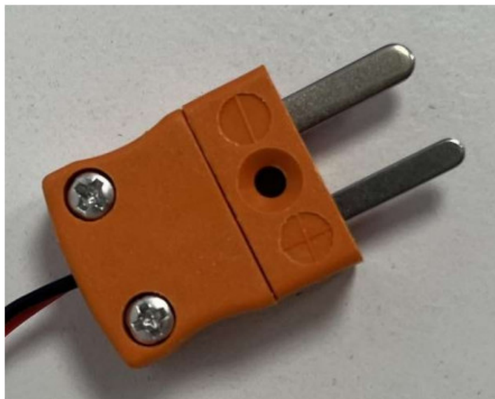
Figure 3 Thermocouple end of Element-B connection cable
