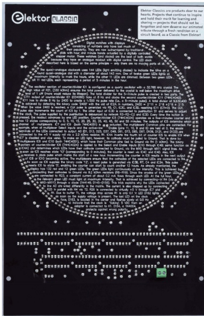
Figure 5: View of back of PCB 240118-1 v1.1. All parts are fitted and soldered.
