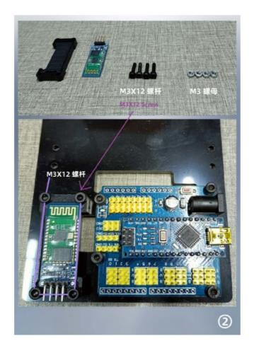
• Then install the bracket with 2x M3X8 screws with nuts
