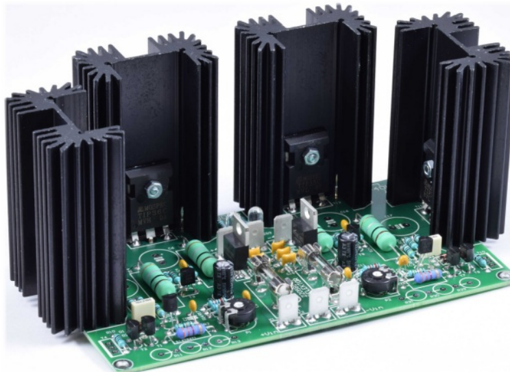
Figure 12: Power transistors fitted to the heatsinks and soldered onto the board.
