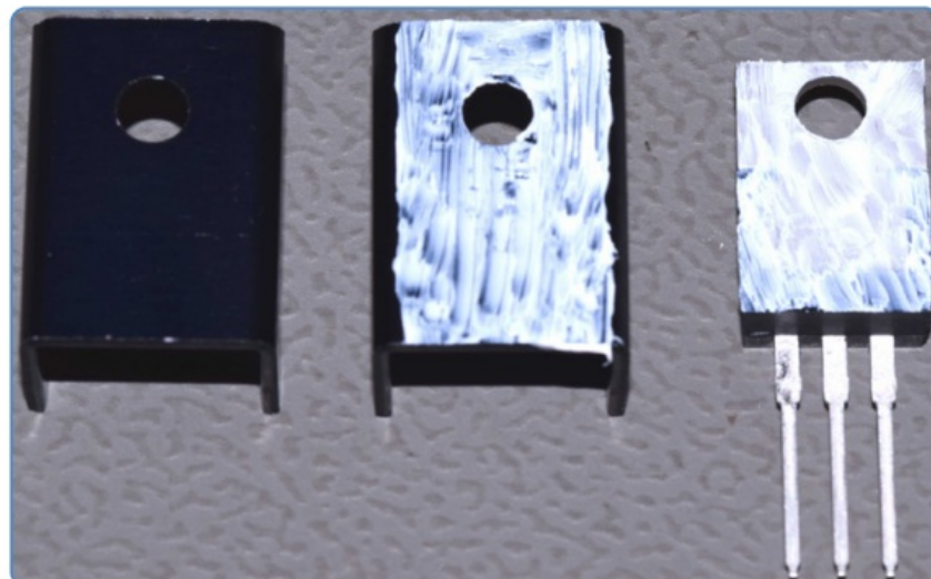
Figure 15: Thermal grease applied to the back of the TO220 transistor and to one of the heatsinks. Now press the backs of the two heatsinks against each other and fasten the transistor firmly to the assembly using the M3 screw, washer, and nut.
