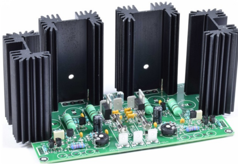
Figure 11: The four large heatsinks soldered onto the board.
