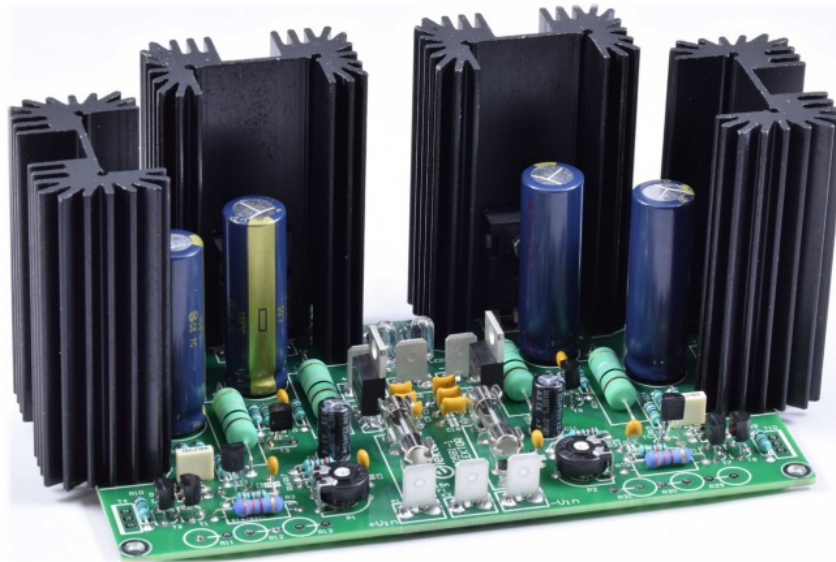
Figure 13: The four large 1000- \mu F decoupling capacitors added.
