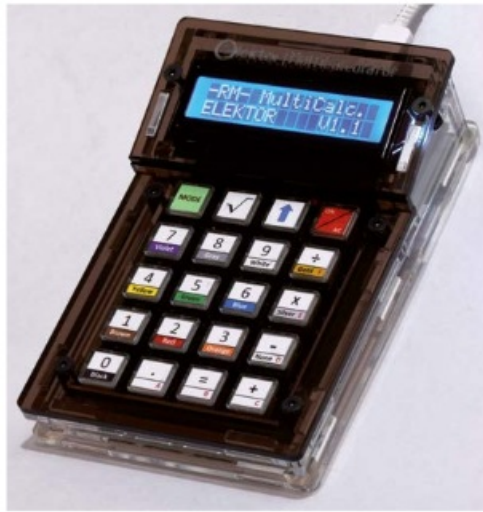
Fig. 25. Assembly of the MultiCalculator is finished. All top panels are installed and fastened.
